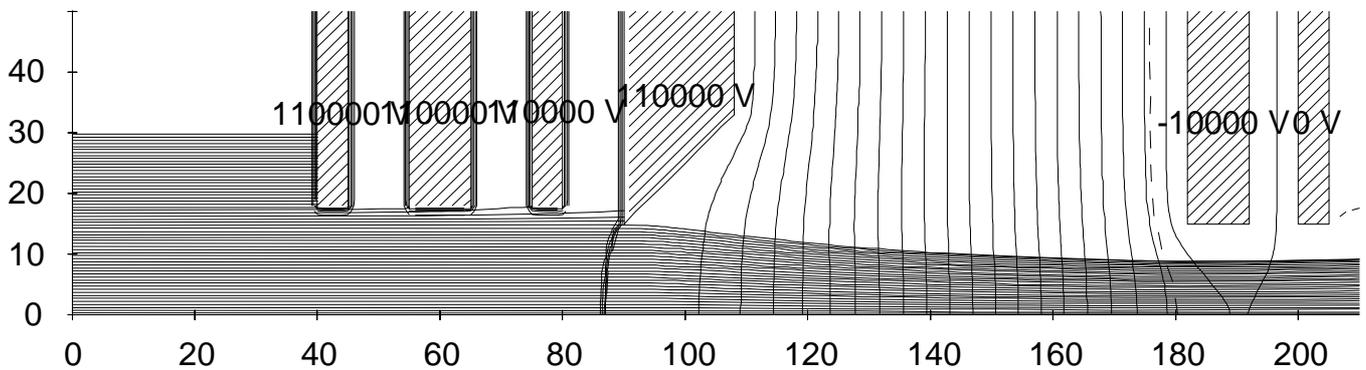
**Operation mode – “shut (-10 kV)”**: Nominal source current would be 200mA – actual source current is cut to 8mA.
